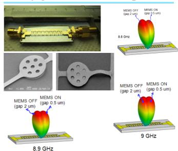
Radiation patterns at 8.8/8.9/9 GHz are tuned from backward in the state of MEMS-All-OFF (state 000000) to the forward in the state of MEMS-All-ON (state 111111). Contact: yluo@iis.u-tokyo.ac.jp
