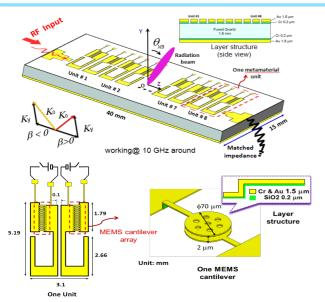
The design consists of 8 periodical J-shaped units which has CRLH property. RF-MEMS switches are used in each CRLH unit to tune the dispersion property
