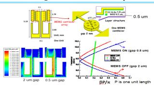
By actuating the RF-MEMS switches, the current of unit is perturbed and redistributed therefore the L, C parameters of the CRLH model are tuned, so that the propagation constant  $\beta$  is controlled by the ON/OFF state of RF-MEMS switches.
