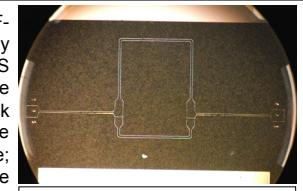
Photo of Monolithic Phase Shifter
